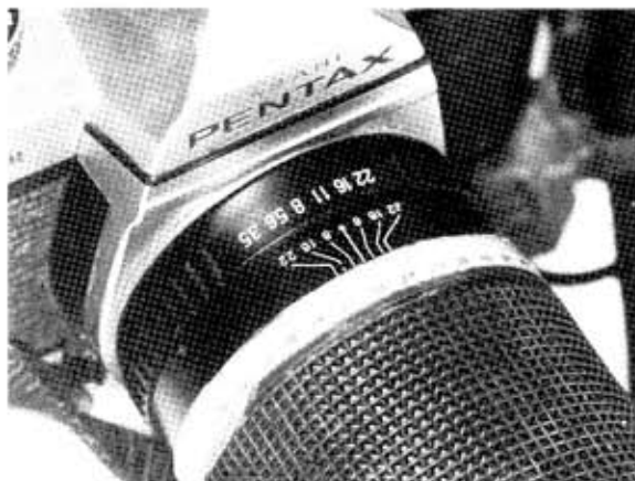
Fig. 2. A millimetre scale taped to the focusing ring so that camera to subject distance can be measured with each photograph.
